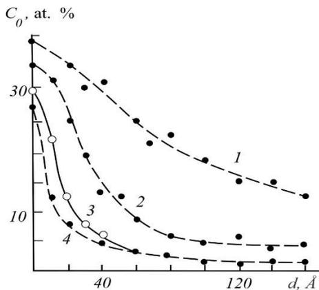
**Fig. 2.** Depth distribution profiles of pure (1) and ion-doped Si (2-4) after contact with air;  $E_0=5.1$  and 0.5 keV (2-4 respectively).
