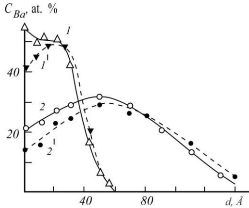
**Fig. 3.** Depth distribution profiles of Ba atoms for Si(111) doped with  $Ba^+$  ions before (1, 2) and after (1', 2') contact with air;  $E_0=0.5$  (1, 1') and 5 keV (2, 2').
