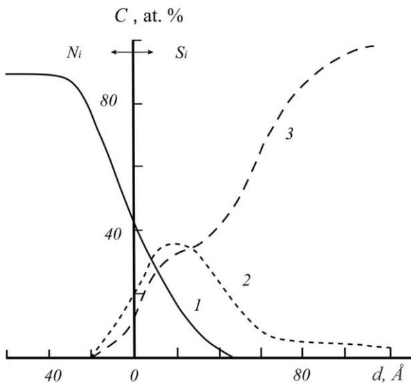
**Fig. 5.** Distribution profiles of (1) Ni, (2) Ba, and (3) Si atoms in the near-boundary region Ni – ion-doped Si; ion energy  $Ba^+$   $E_0=0.5$  keV.
