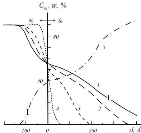
**Fig. 4.** Depth distribution profiles of Ni atoms of (1) pure single-crystal and (2) amorphous silicon and silicon doped with  $Ba^+$  ions with an energy of 5 (3) and 0.5 keV (4); 5-distribution profile of Si in the near-contact region Ni – pure Si (111).
