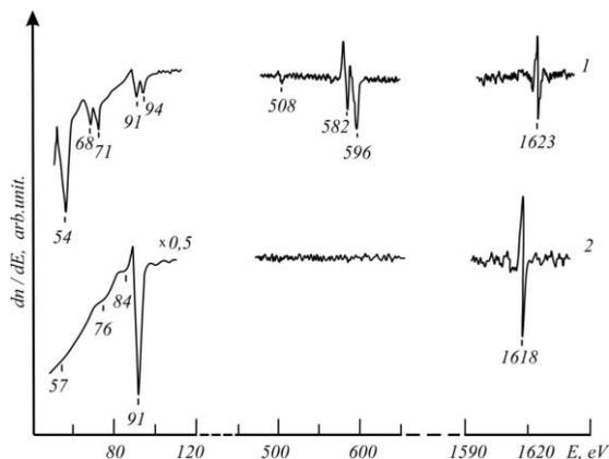
**Fig. 1.** Auger spectra of pure and ion-doped Si; 1 –  $Ba^+ \rightarrow Si$ , 2 – Si(111);  $E_0=0.5$  keV;  $D=6 \cdot 10^{16} \text{ cm}^{-2}$ .
